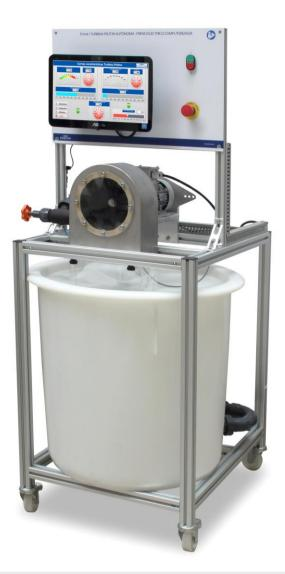
The TH 04.1 model is an advanced, scaled-down Pelton turbine (or action turbine) simulator, specifically designed to facilitate detailed study and real-time visualization of the behavior and dynamic properties of such turbines.
